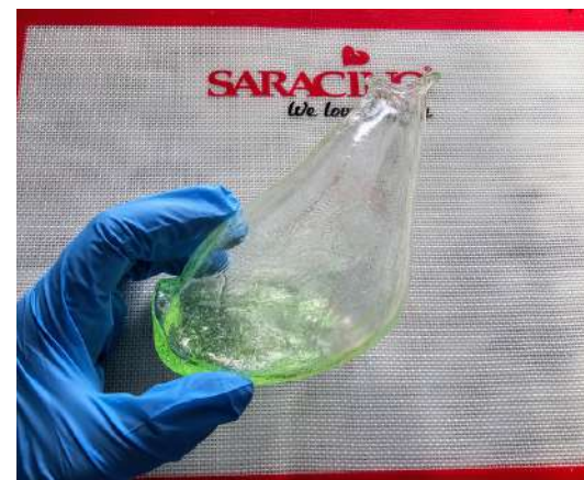
STEP 51 Note, I ended up not using this vase as the neck wasn't quite right for what I wanted. To open the vase top, gently heat for a second or 2 with your blow torch on a low temp and use the metal rod on the pump to push the inside edge of the vase outwards. Go around the entire rim until you have widened enough. Heat the edges cautiously.
